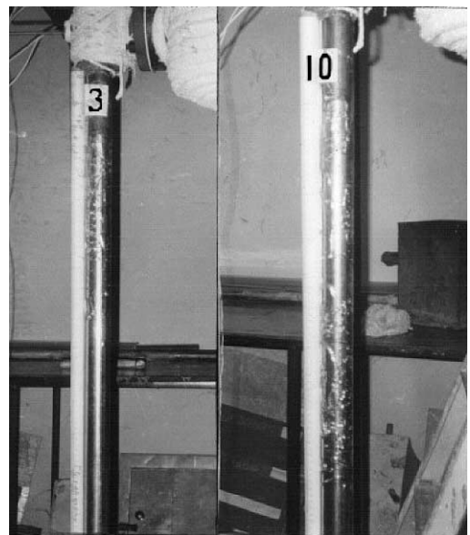
Plate 3. Effective boiling zones at a heat flux of 9.5 kW/m 2 with S = 100% (left tube) and S = 75% (right tube).
